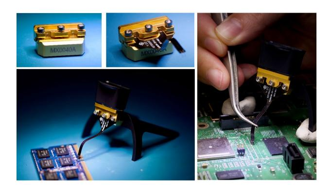
The N5445A browser head (30 GHz) is the best choice for quick general-purpose troubleshooting of differential signals with its z-axis compliance and variable spacing from 20 mil to 125 mil (or 0.5 mm to 3.1 mm). The span between the signal tips is easily adjusted with a thumb wheel on the browser. Integrated LED lighting at the tip illuminates the probing area for better visibility. Order N5476A for replacement browser tips (set of 4).
