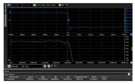
8.8ps edge is measured with InfiniiMax 4 probing solution
